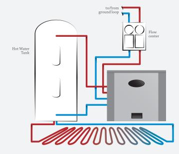
During the heating cycle, the fluid circulates through the loop extracting heat from the ground. The heat energy is transferred to the geothermal unit. The unit compresses the extracted heat to a high temperature and delivers it to your home through a radiant heat system or by a duct system when paired with an air handler.
